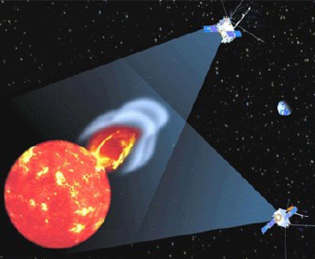
The 2 STEREO-spacecraft observe the Sun simultaneously. For observing (plasma on) magnetic field lines, we use mainly EUV-images from STEREO/SECCHI.
