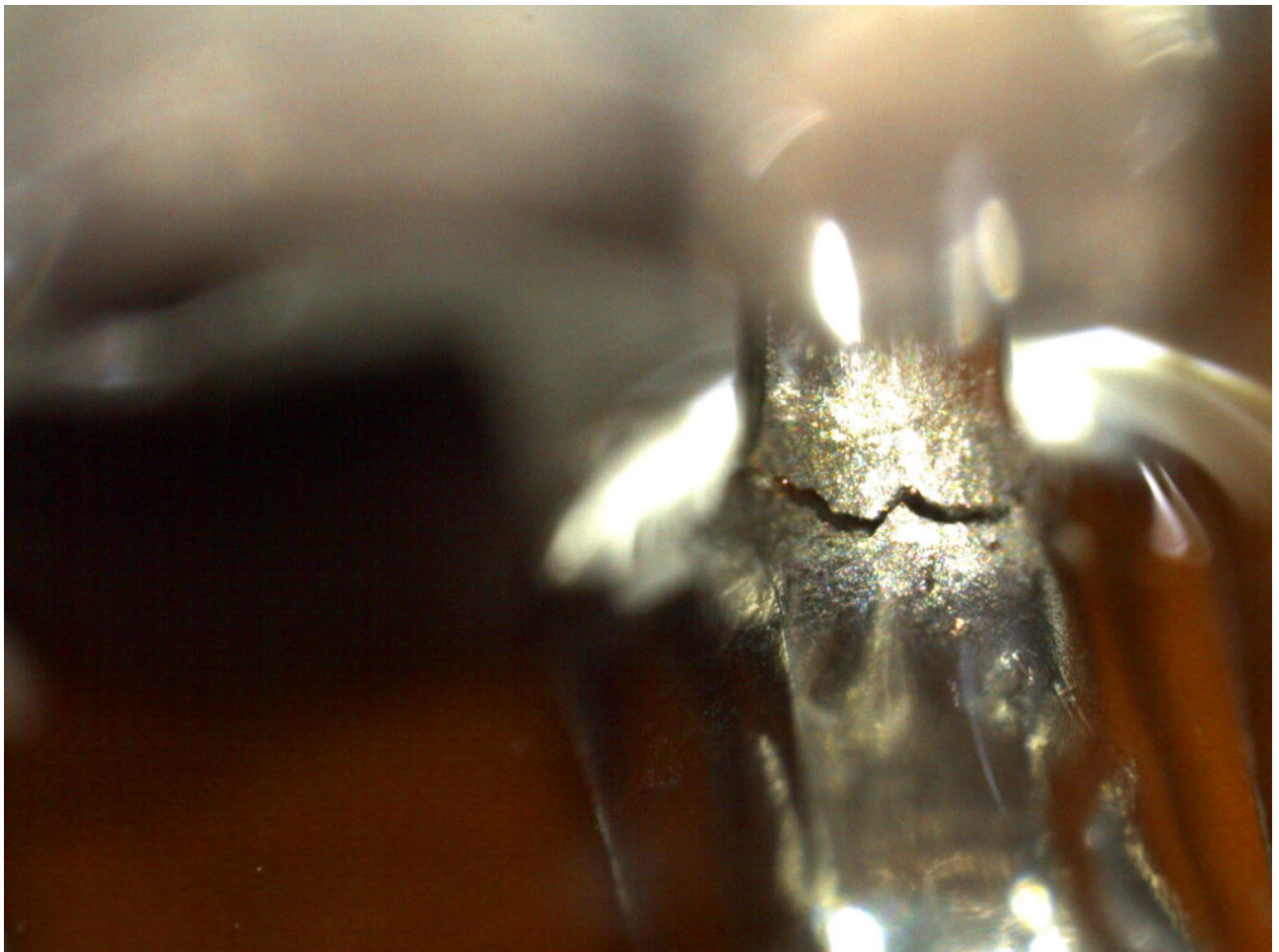
Abb 4 Crack at Capacitor C309 detail
