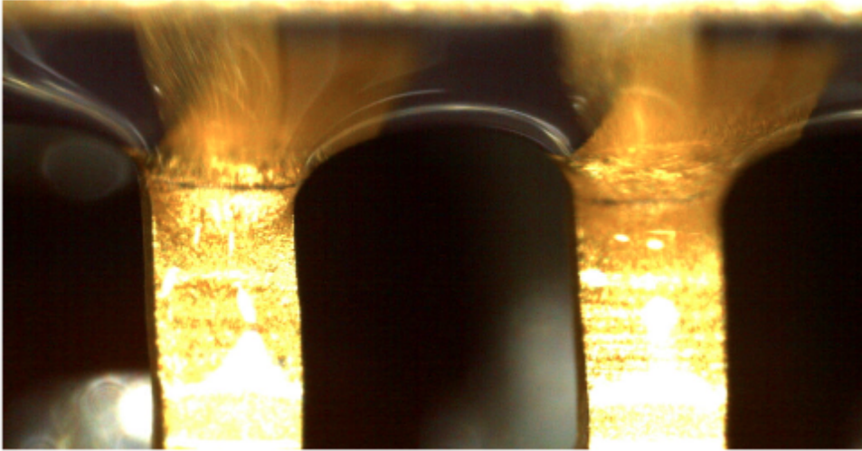
Abb 6 Crack on Pin 1 &2 at IC301 detail 01
