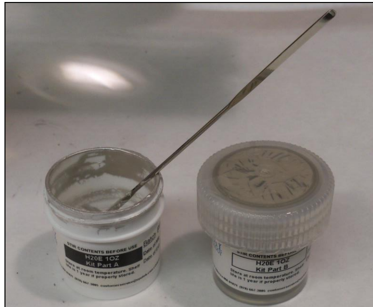
Figure 4.1-1 Part A & B of H20E. Micro spatula used for taking material out of container.
