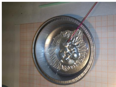
Figure 3.1-2 Aluminium bowl with mixed H20E, AWG24 PTFE-coated single-wire used as dosing tool.
