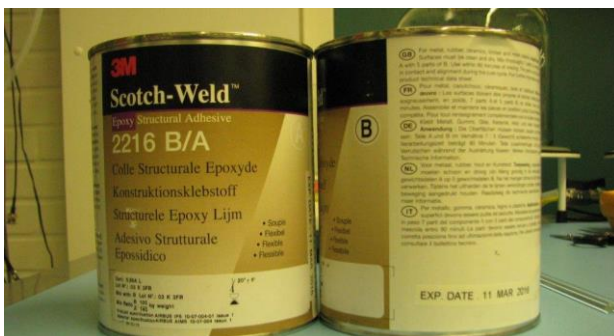
Figure. 5.2-1: Pots with part A and part B of 3M Scotch-Weld
