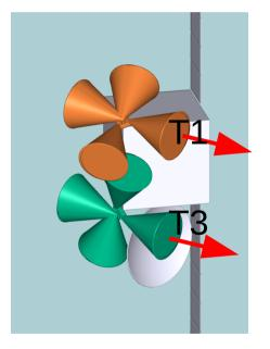
T1 and T3 point approximately in the direction of the nominal Parker spiral (45°). T2 and T4 point in the only directions which could be accommodated.
