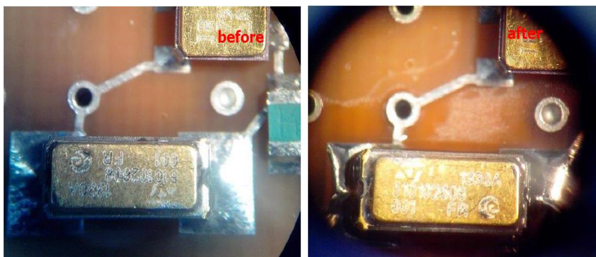
Figure 4 Diodes before and after rework
