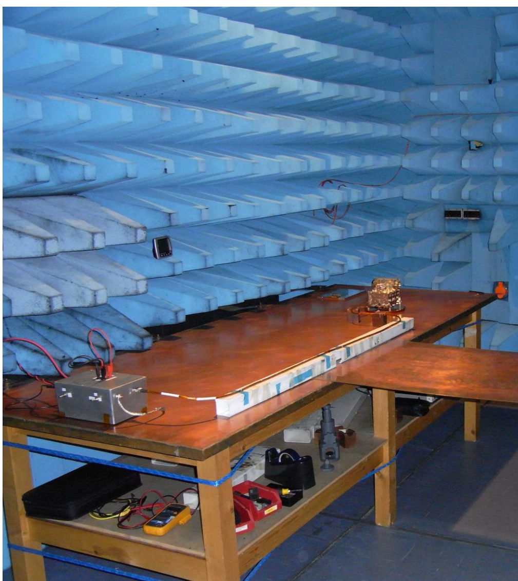
Figure.1 General EMC Test Setup.
