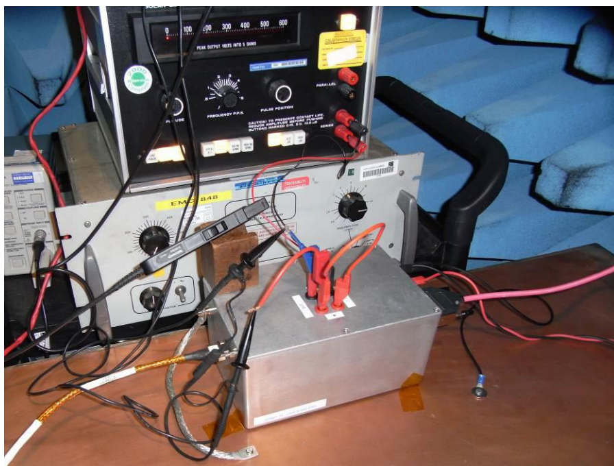
Fig 12. 150ns Transient set-up (-VE Line)
