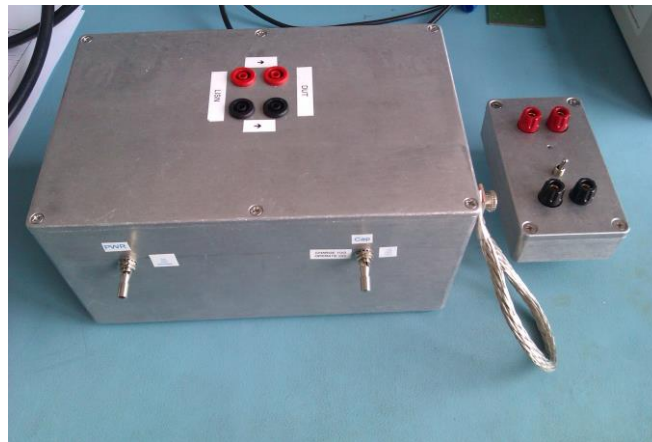
Fig. 5-2. LISN used for STEP EM EMC test campaign.
