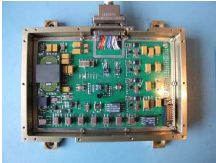
Low Voltage Power Supply inside the corresponding housing part
