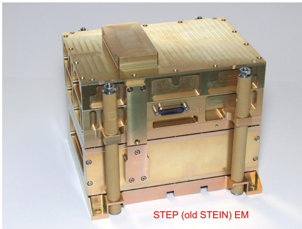
Fig. 4-7-1. STEP EM for unit level EMC test campaign.
