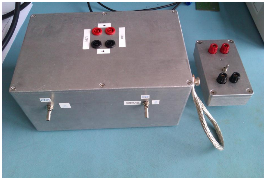
Fig. 5-2-2. LISN used for STEP EM EMC test campaign.
