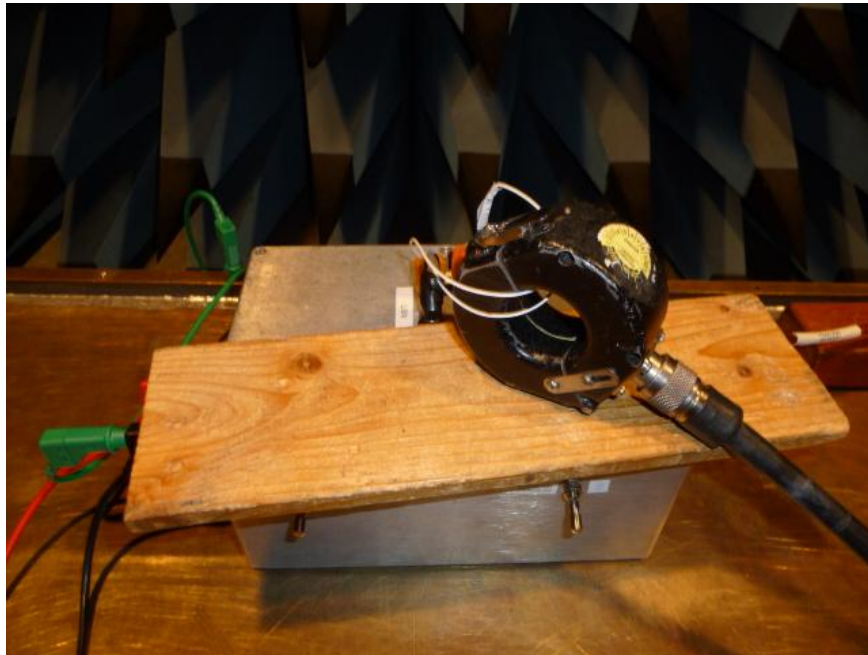
Fig. 30: Conducted emission on power leads, common mode, 30 Hz to 100 MHz, frequency domain(6.3)
