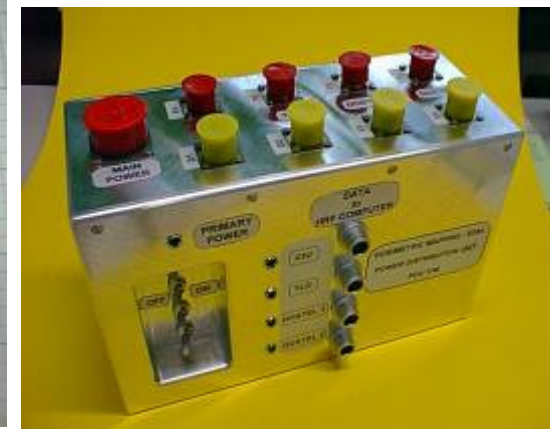
Power Distribution Box
