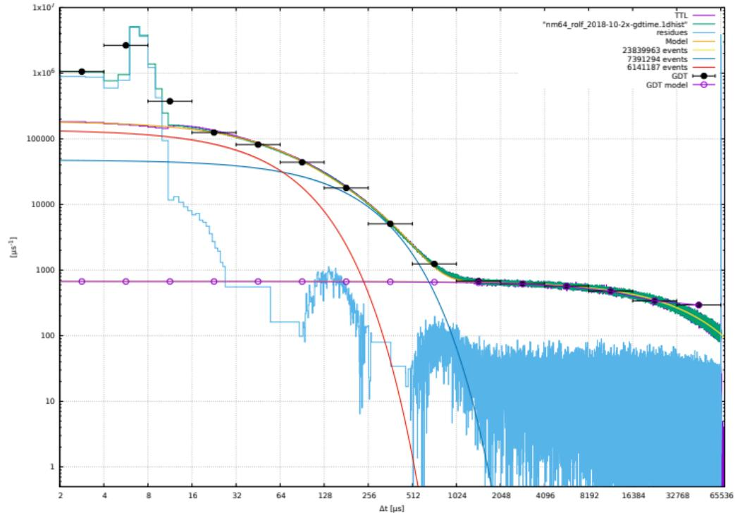
Analysis of the last six  $\Delta$ -time counters may yield an alternative count rate value, independent of instrumental effects like pileup, multiple-hits.
