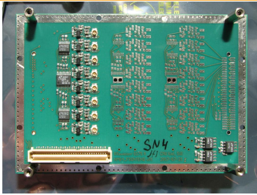
The NM64\_FRONTEND board receives and conditions the outputs from the counter tube preamplifiers.
