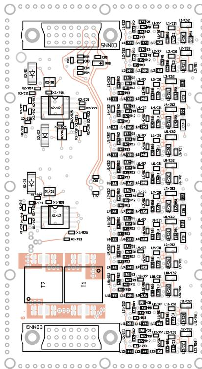
There are 5 different drill sizes used in this layout, 462 holes total
