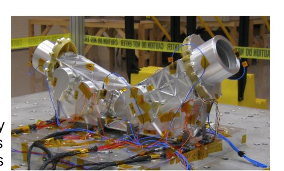
SIS EM during vibration testing.
