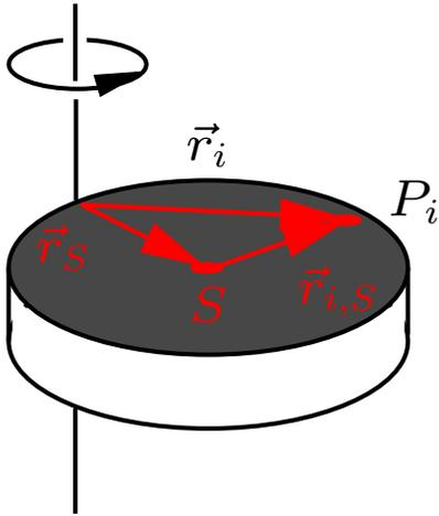
$$\begin{aligned}\vec{r}_i &= \vec{r}_S + \vec{r}_{i,S}, \\ r_i^2 &= r_S^2 + r_{i,S}^2 + 2\vec{r}_S \cdot \vec{r}_{i,S}, \\ \sum_i m_i r_i^2 &= \sum_i m_i r_S^2 + \sum_i m_i r_{i,S}^2 + 2\vec{r}_S \cdot \sum_i m_i \vec{r}_{i,S}, \\ &= Mr_S^2 + J_S + 2\vec{r}_S \cdot \sum_i m_i \vec{r}_{i,S} = Mr_S^2 + J_S,\end{aligned}$$
