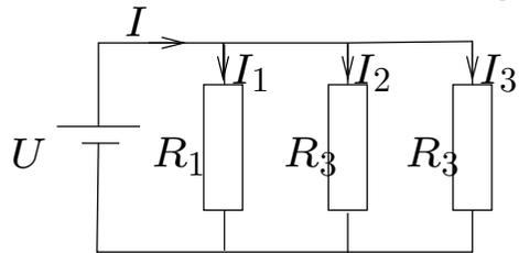
$$\frac{U}{R} = I = I_1 + I_2 + I_3 = \frac{U}{R_1} + \frac{U}{R_2} + \frac{U}{R_3}$$
