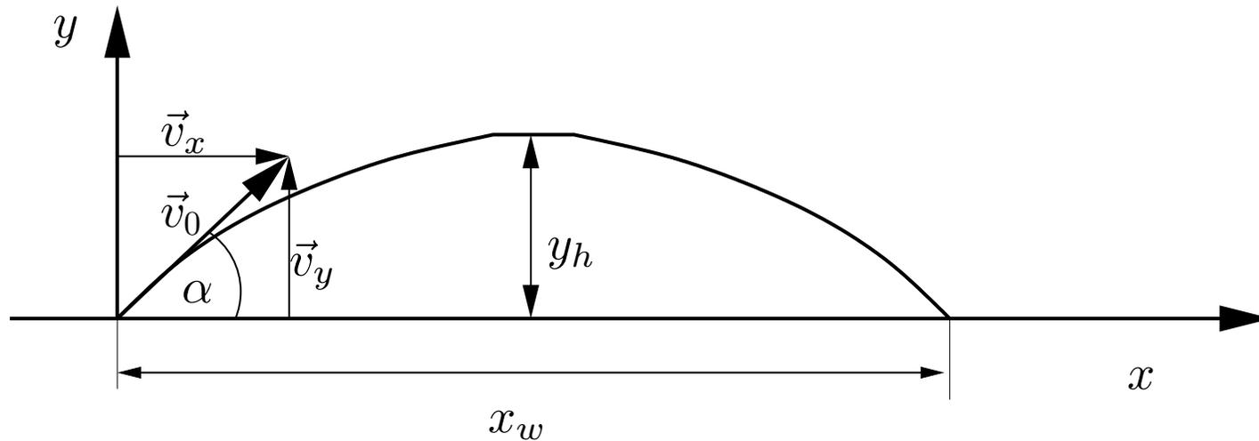
$$v_x = v_0 \cos \alpha; \quad v_y = v_0 \sin \alpha - gt$$
