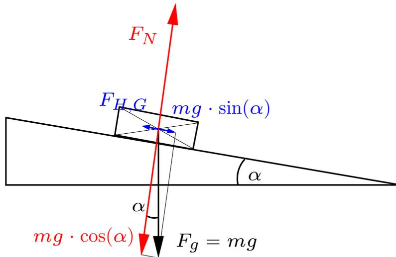
$$\begin{aligned}\sum \vec{F}_i &= mg \cos \alpha_{H,G} + F_N + mg \sin \alpha_{H,G} + F_{H,G} = 0 \\ \sum F_{\perp} &= mg \cos \alpha_{H,G} + F_N = 0 \\ \sum F_{\parallel} &= mg \sin \alpha_{H,G} + F_{H,G} = 0\end{aligned}$$
