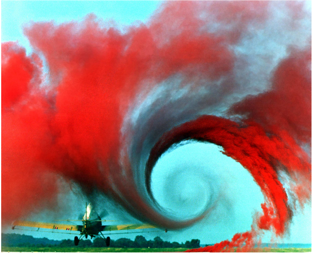
Figure 7.1: The air flow from the wing of this agricultural plane is made visible by a technique that uses colored smoke rising from the ground. The swirl at the wingtip traces the aircraft’s wake vortex, which exerts a powerful influence on the flow field behind the plane. The vortex dissipates after some time, thereby driving turbulence via a turbulent cascade. Source: Wikipedia/NASA-Langley photo-ID EL-1996-00130.
